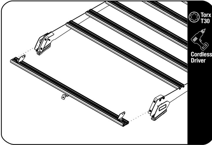
Secure assembly 2.3 to the front two bottom holes on the foot rails using the fasteners removed in step 2.1. Fully tighten.
