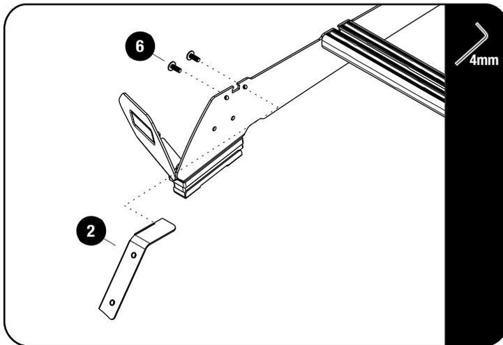
Secure the Wind Fairing Side supports LH / RH (Item 2) to the foot rails top holes as shown using M6x16 Flange Button Heads (Item 6).
