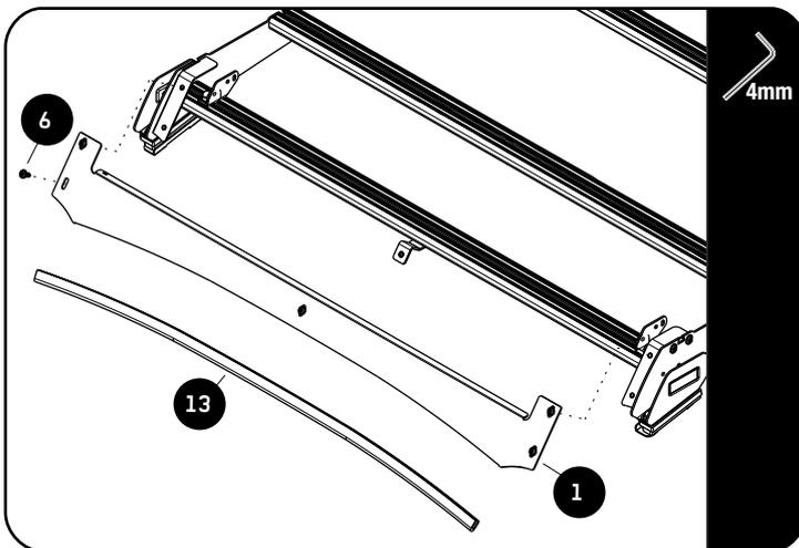
Fit the Wind Fairing Rubber (Item 13) to the Light Bar Wind Fairing (Item 1). Using the notched section as a guide, trim if needed.
