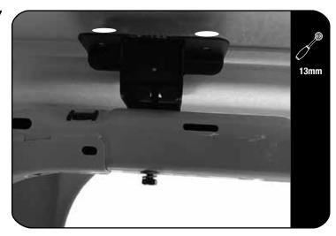
Secure the rear Inner Bracket (Item 6) using a M8 x 100 Hex Bolt, M8 SS Spring Washer and M8 x 19 x 2SS Flat Washer. (Items 15, 16 & 17) As shown.
