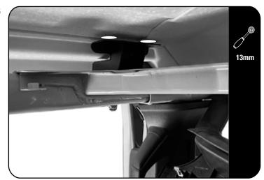
Secure the front Inner Bracket (Item 6) using a M8 x 100 Hex Bolt, M8 SS Spring Washer and M8 x 19 x 2SS Flat Washer. (Items 15, 16 & 17) As shown.
