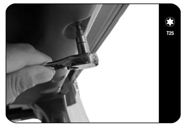
Looking at the roll cage at the rear passenger door, remove the plastic trim covers located on the inside of the roll bar as
