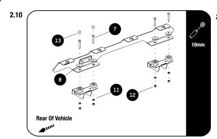
Place the Foot Rail (Item 1) onto the Spacers and secure using M6 x 40 Hex Bolts, M6 x 30 x 2 Flat Washers, M6 x 12 x 1SS Flat Washer and M6 Nyloc Nuts (Items 7, 8, 11 & 12) as shown. Do this on both sides of the vehicle.
