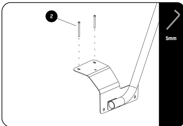
Apply a small bead of Thread Lock on the thread around the tip of the M6x80 Cap Screws (Item 2).
