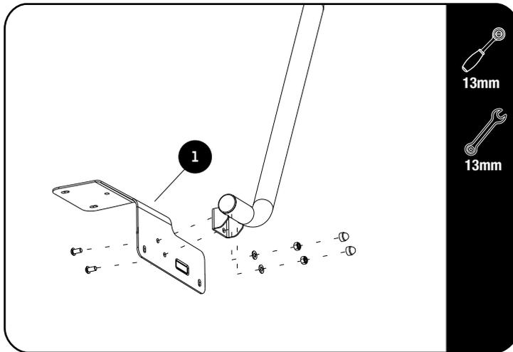
Assemble the LH Cowling Bracket (Item 1) to the LH Support Arm supplied the FAJL004 using two M8x16 Button Head Screws, two M8 Flat Washers and two M8 Nyloc Nuts (Fasteners also supplied with FAJL004).
