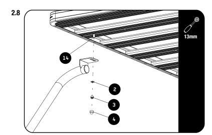
Fit your Roof Rack to the Front Support Arms using M8x20 Hex Head Bolts, M8 Flat Washers and M8 Nyloc Nuts (Items 14, 2 & 3) as shown.
