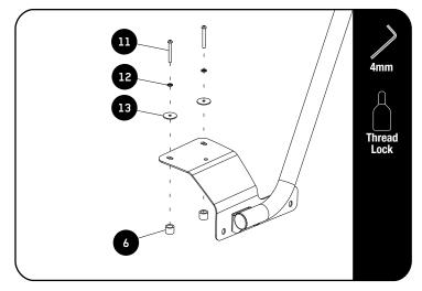
Apply a small bead of Thread Lock on the thread around the tip of the M6x50 Button Head Screws (Item 11).
