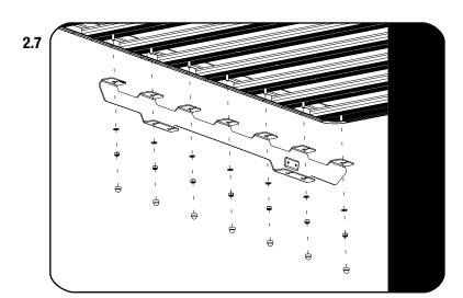
Fit your Roof Rack to the Inner and Middle Support Brackets.
