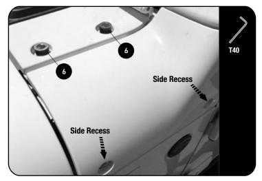
Using a T40 Torx Wrench, remove the four bolts holding the Corner Cover in place.
