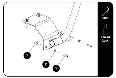
Place two Spacers 19x12x12 (Item 7) into the two side recesses shown in 2.2, between the Front Support Arm and the Corner Cover.
