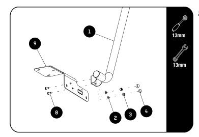
Assemble the LH Front Support Arm
