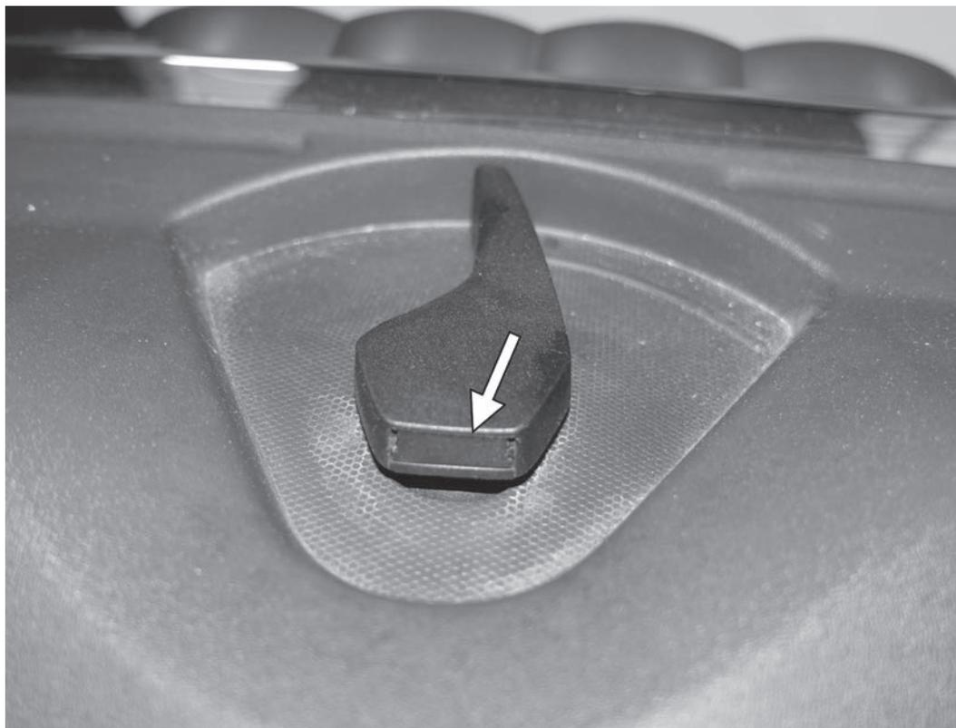
1) Raise the hood and remove the hood latch by pressing in on the small button on the back of the latch, and then lifting the latch up and away from the car. Be sure to not close the hood with the latch removed!
