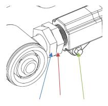
Tighten this nut (blue arrow) against other adjuster (red arrow). Tighten Locking bolt (green arrow)
