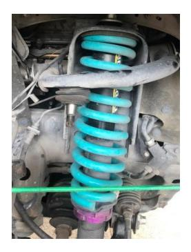
3. Set up arm as per below picture for installation. This is a good general starting point for normal alignment. Set the base of UCA to the base of eye at 39mm. Lock of the arm nuts against each other and tighten the locking bolt in second picture. With this setting it will give you the ability to set the alignment with the bottom lower control arm.
