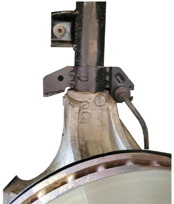
**CHECK IF ORIGINAL BOLT IS ABOVE FLANGE OR THROUGH HOLE. FIT THE SAME AS ORIGINAL**
