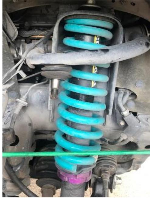
3. Using OE bolts and supplied bush washers loosely bolt the Dobinsons UCA into the OE chassis mounts, using the Left and Right arms. Fit the supplied washers to the outside of the arms (outsides of either end bushes). This should look like the OE fitment.
