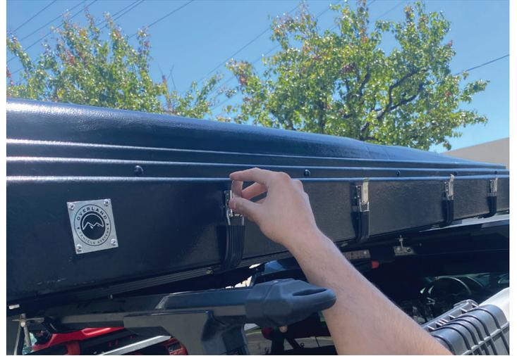
6. Pull down the straps, and securely fasten the fastening clips and reinforced straps.
