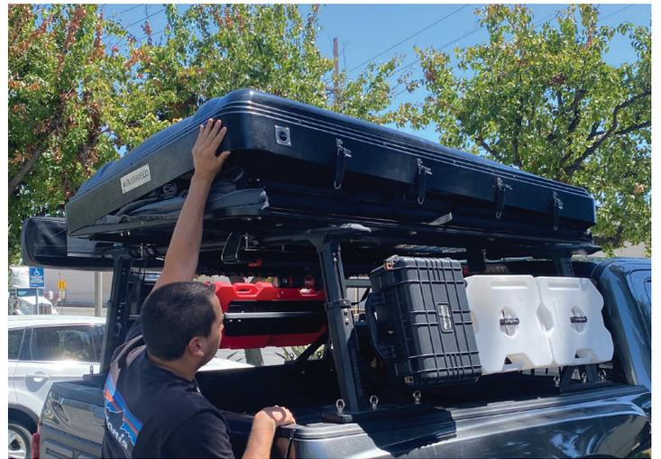
7. The fastening clips and reinforced straps keep your tent closed. ALWAYS make sure that the hard shell is completely closed and the straps are securely fastened before driving.
