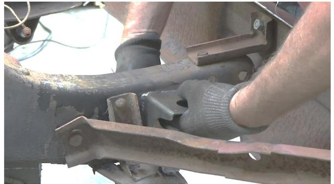
On the bottom of your core support mount, use a 15mm socket to screw in the two 25mm bolts and nuts.
