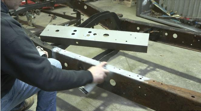
Push the part onto the frame while using the frame holes to help with alignment.
