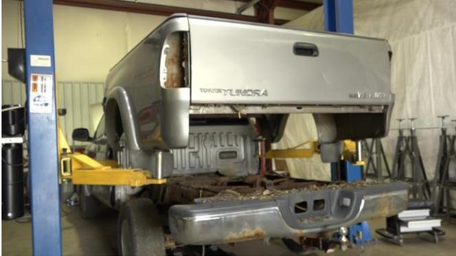
Hold the part up to the frame and take note of its coverage. Mark out your cleaning and grinding area.
