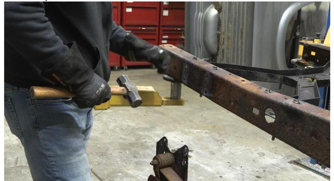
Clean and grind the frame free of rust and debris, revealing bare metal.
