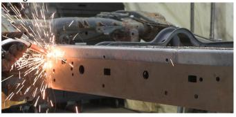
Remove any potential fire hazards from the work area. Following proper welding procedures, tack weld the part onto the frame before welding it on fully. Weld 100% around all edges.
