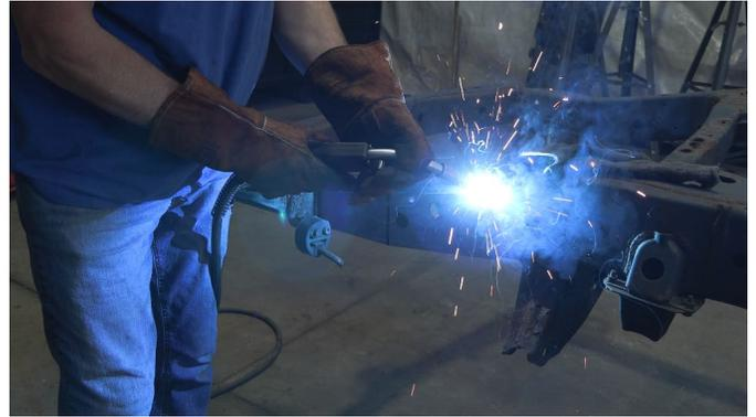
Followed by pushing the rear section up and aligning that area's frame holes, and tac welding it.
