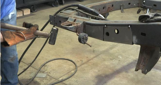
Remove any potential fire hazards from the work area. Following proper welding procedures, tack weld the part onto the frame before welding it on fully. Weld 100% around all edges.
