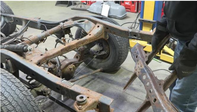
Then, grind down the mounting areas free of rust and debris, revealing bare metal.
