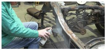
Clean the frame free of rust and debris, revealing bare metal.
