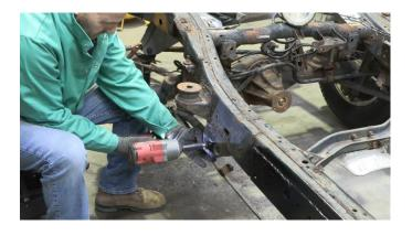
Draw a line ¾ inch above the frame and cut along it to remove the bottom of the frame.
