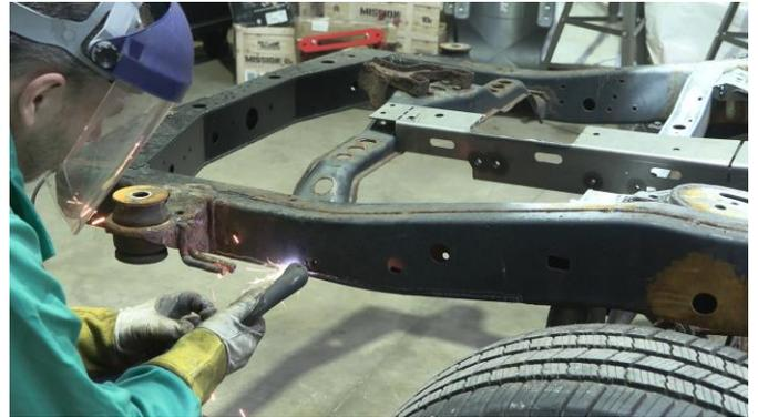
Then, grind down the zones free of rust and debris, revealing bare metal.
