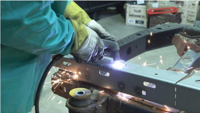
Hold the part up to the frame and mark off its coverage. Bend the opening on your rear frame section to create the contour of your frame. Then, mark your cutline  $\frac{3}{4}$  inch above the bottom of the frame.
