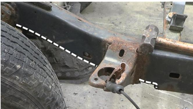
You can choose to leave the existing body mount or replace it with a new one. If you are keeping your old body mount, cut along the perforated line.
