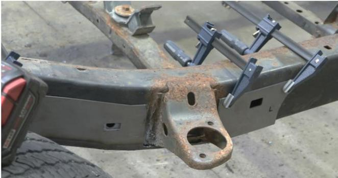
Remove any remaining potential fire hazards on both the vehicle and surrounding area. Following proper welding procedures tack weld the part onto the frame before welding the part on fully. 100% weld around all edges.
