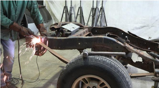
Grind the work area free of rust and debris, revealing bare metal/ followed by coating the work area with a weld through primer to help prevent against further rust development.
