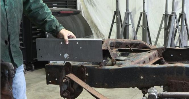
Our part features removable/perforated plates to allow the part to go around the spare tire crossmember's retaining rivets. If you are not replacing the crossmember, remove these plates as needed.
