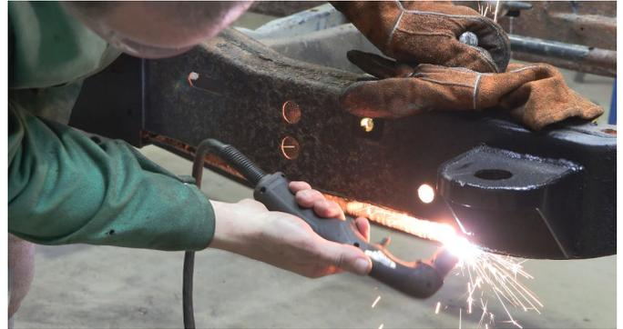
Grind the frame rail free of rust and debris, revealing bare metal.
