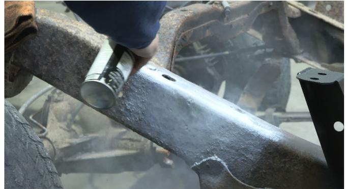
Referencing the mounts on the opposite side of the vehicle, measure 12 $\frac{3}{4}$  inches from bolt hole center to center and 3 inches up from the top of the frame, and mark off the install location.
