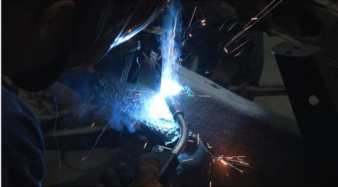
Remove any potential fire hazards from the work area. Following proper welding procedures, tack weld the part onto the frame before welding it on fully. Weld 100% around all edges.
