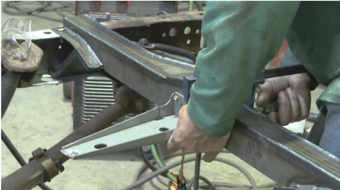
With the supplied M10 hardware, use a 13mm socket to bolt the spare tire plate to the frame
