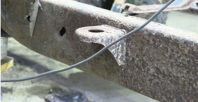
Coat the work area with a weld through primer to help prevent against further rust development.
