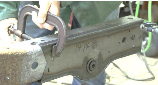
Following proper welding procedures, tack weld the part into place before welding it on fully. Weld 100% around all edges.
