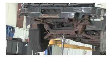
Using an 18mm socket, remove the body mount bolt and bushing.
