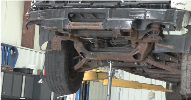
Using a screw driver, push off the shown tabs and remove the break lines.
