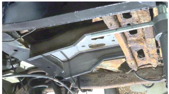
Following proper welding procedures, tack weld the part into place before welding it on fully.
