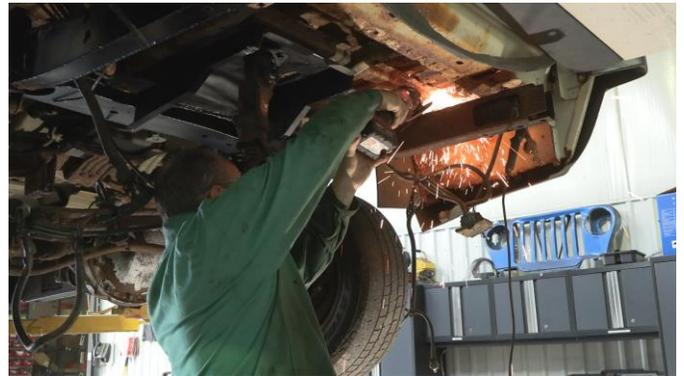
Coat the part and work area with a weldable primer to help prevent against rust development.
