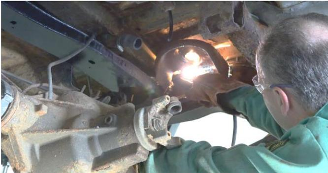
Grind down the frame free of rust and debris, revealing bare metal.
