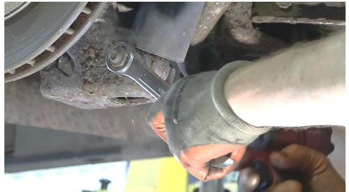
Remove your bump stop. This makes the part easier to weld on without the bump stop getting in your way.
