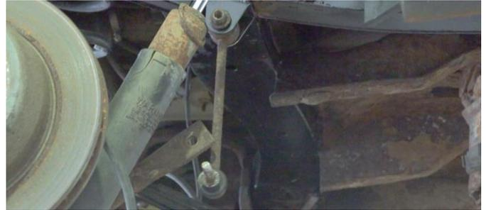
Using a 21mm socket and wrench, remove the bottom shock bolt, along with the shock. This relieves the spring so we are able to move it out of the way of our work space.
