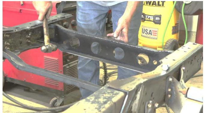
Once in place, use a 14mm socket and 15mm wrench to screw in the included M10 hardware on the top and bottom of your frame rail.
