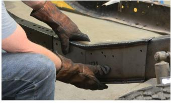
If you purchased part number RB7359 / RB7372, install the mount with the included hardware with a 14mm and 13mm socket and wrench.
