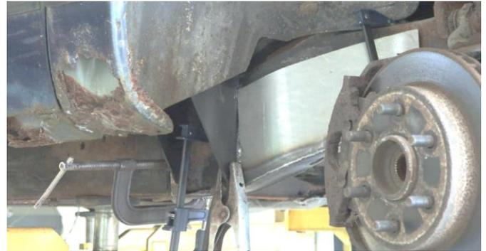
Following proper welding procedures, tack weld the part onto the frame before welding it on fully. Weld 100% around all edges.
