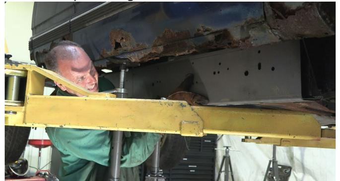
Tac-weld the part and confirm its alignment before completely welding it onto the frame.
