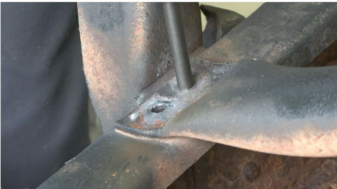
Clean and grind the area free of rust and debris, revealing bare metal. Coat the area with a primer to help prevent against further rust development.
