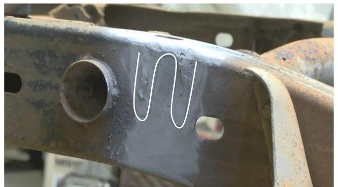
Remove any potential fire hazards from the work area. Following proper welding procedures, tack weld the part on before welding it on. 100% weld around all edges.
