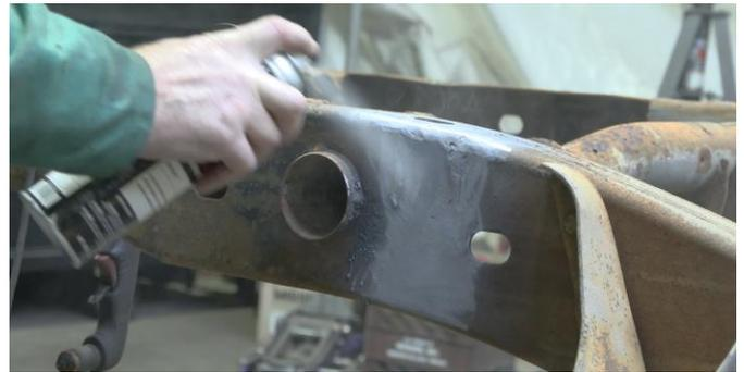
Hold the part up to the frame and mark off its coverage using a paint marker.
