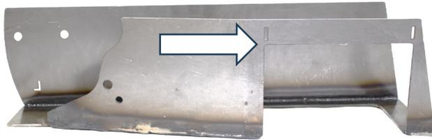
Grind the work area free of rust and debris, revealing bare metal/ followed by coating the work area with a weld through primer to help prevent against further rust development.
