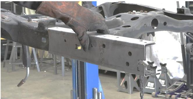
Following proper welding procedures, tack weld the part onto the frame before welding the part on fully. Weld 100% around all edges.
