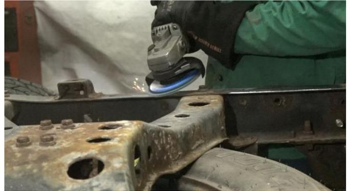
Clean the frame free of rust and debris, revealing bare metal.
