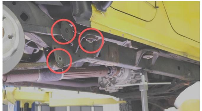
With a 21mm socket, remove the bolts securing both your upper and lower control arms, followed by an 18mm socket to remove the nearby body mount bolt and bushing.
