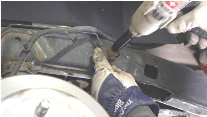
With a 5/8 socket, remove the 2 bolts from each sway bar bracket to relieve tension on the axle.
