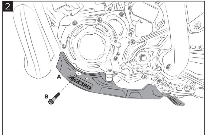
**Secure the Skidplate (A) to the frame by tightening the bolts (B) on both sides.**
