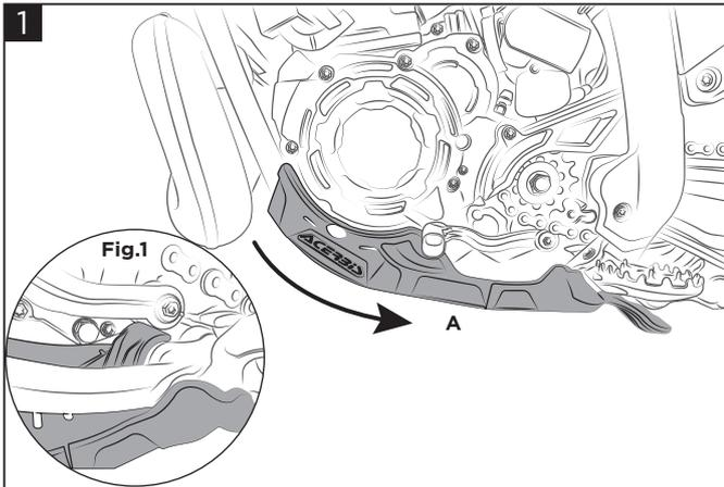
**With force, push the skid plate (A) back towards the rear as indicated with the arrow. Make sure that the hook on the back of the skid plate is securely placed up and over the rear frame support tube (figure 1).**
