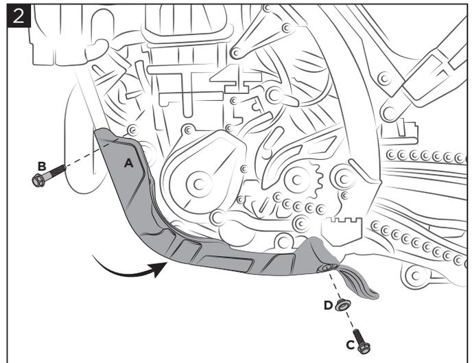
**Position the Acerbis skid plate (A) and fix it using the supplied screws (B), the bushings (D) and the second screws (C).**
