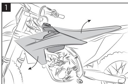
**Remove the original side panels and saddle.**
