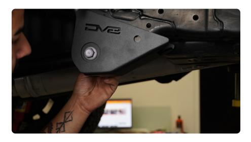
STEP 6 | Using the provided M12 bolts, install the bolt into the upper mounting hole of the skid plate though the hole on the mount.
