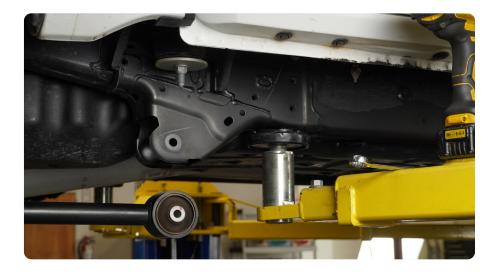
STEP 4 | Place the skid plate towards the front of the trailing arm, slide the skid plate up and back ensuring the skid plates welded spacer sits in front of (towards the front of the vehicle) the lip thats on the trailing arm mount (red arrow).
