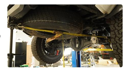
STEP 2 | Use a 19mm socket and wrench to remove the trailing arm bolt and nut.
