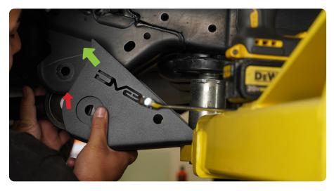
STEP 5 | With the skid plate in position loosely secure the skid plate in place using the factory hardware.
