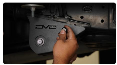
STEP 7 Using a 18mm socket and 19mm wrench, tighten the upper bolt until secure.
