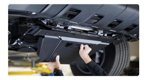
STEP 7 Use the (4) provided M12 hardware with (1) flat washer and (1) split washer each bolt to loosely secure the front of skid plate (and recovery hooks) to the vehicle.
