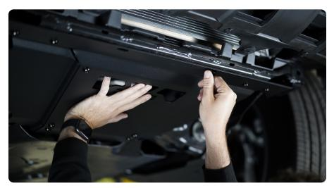
STEP 8 | Use a #5 Allen tool to secure the (2) rear M8 mounting bolts.
