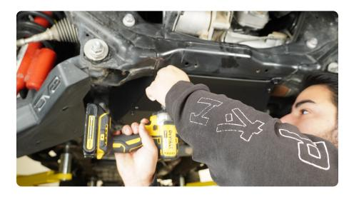
STEP 10 | Lift up the DV8 Front Skid plate aligning the front mounting holes with the recovery hook threaded holes while sandwiching SPTT1-09 between the front cross-member and front skid plate.
