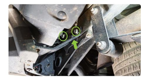
STEP 5 Use a 21mm socket to remove the (4) bolts that secure the tow hitch/bumper support to the frame rail.
