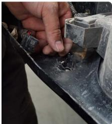
STEP 13 | Start assembling the DV8 bumper by first installing the bumpers mounting nut clips.
