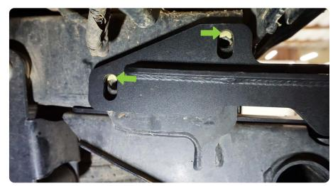
STEP 27 | Use a small sanding wheel or drill bit to remove the material and slot the mounting holes on each side.
