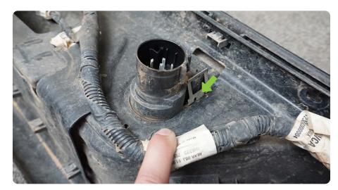
STEP 11 | Use a trim clip tool to free the sensor/light harness from the bumper.
