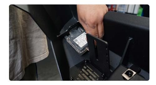
STEP 18 | Use the provided retaining bracket and M6 hardware, 10mm and #4 Allen tool to secure the Blind Spot sensor in place.
