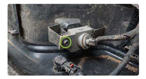
STEP 10 | Use a trim clip tool to remove the trailer light socket. Depress the clip on each side and press the trailer socket our the front of the bumper.
