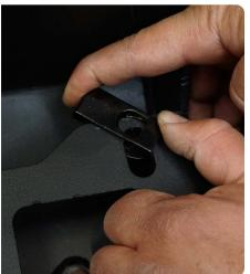
STEP 14 | If your vehicle is back up sensor equipped, remove the DV8 sensor plugs by pressing them out through the front of the bumper.
