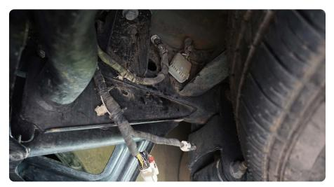
STEP 3 | Disconnect the trailer light socket.
