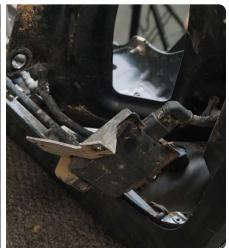
STEP 8 | Remove the back up sensors by gently prying apart the sensor bezel tabs and pressing the sensor out from the front side.
