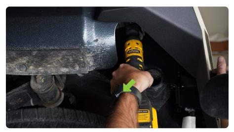
STEP 30 | Reconnect two plugs removed during the uninstall.
