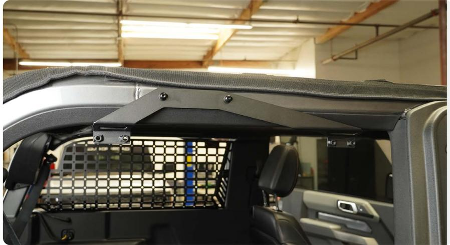
**STEP 14** | Mount the rear base bracket using the factory hardware ensuring the bracket is fully adjusted towards the vehicles trunk area.
