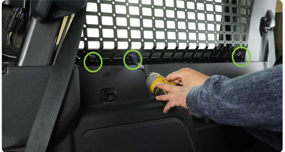
**STEP 9** | Loosen but do not remove the (4) roll-bar brackets M8 Allen head bolts on each Molle panel using a #5 Allen tool.
