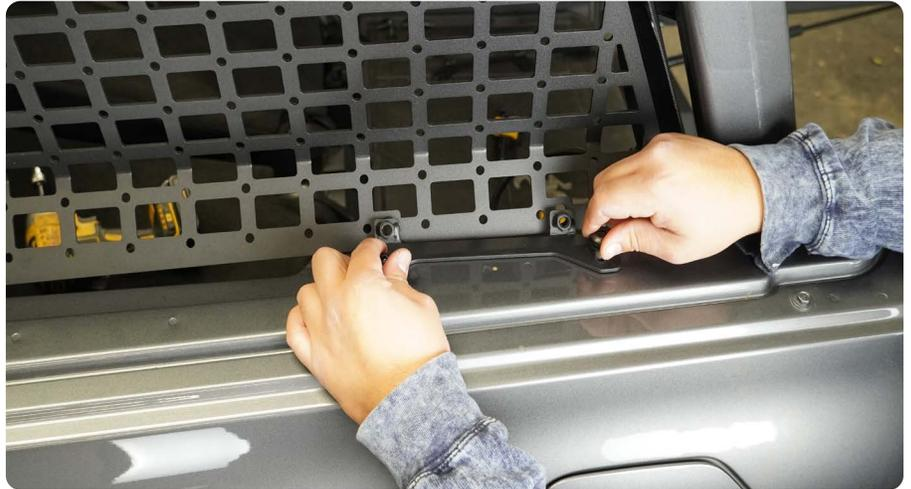
**STEP 12** | Use the molle panels M8 allen head hardware and a #5 Allen tool to secure the panel back to the mounting bracket.
