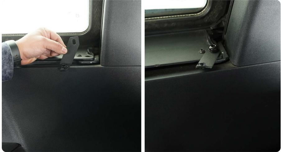
**STEP 5 |** Using the provided M8 hardware and a #5 Allen tool, loosely secure the roll-bar mounting bracket as shown.
