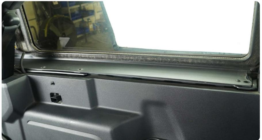
**STEP 3** | Using the factory hardtop hardware, molle panels rear base bracket.
