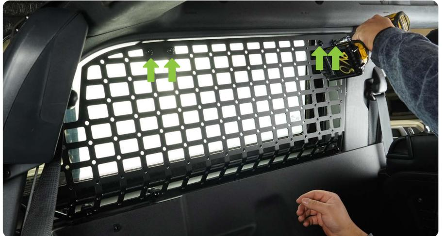
**STEP 10** | With the roll-bar brackets hardware loosen and the base brackets hardware removed you can now reach under the DV8 molle panel to gain access to the hardtop mounting hardware to remove the factory hardtop.
