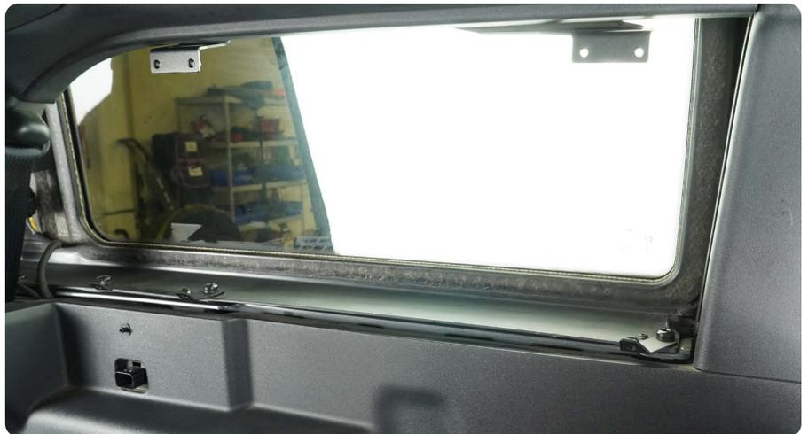
**STEP 7 |** Use the provided M8 hardware and an #5 Allen tool to secure the DV8 molle panel to the provided mounting brackets.
