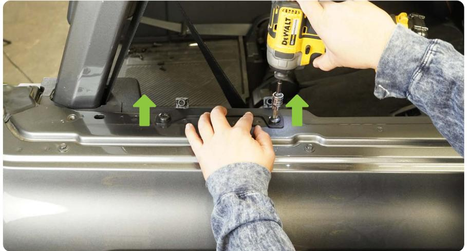
**STEP 15** | Loosely mount the front base mounting bracket behind the vehicles "B" pillar using the factory hardware.
