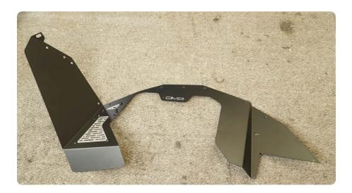
STEP 6 | Place the mid sized panel with threaded rivnuts as shown, with the riv-nuts lip on the back side of the base panel.
