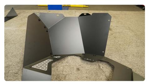
STEP 8 | Align the large sized panel with the base panel and mid panel as shown. Ensure the riv-nuts lip is placed behind the mid panel and base panel.
