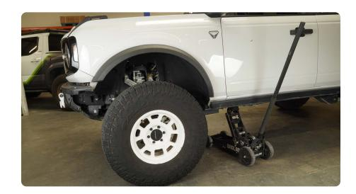
STEP 2 | Using a small Philips head screw driver and a trim clip tool, remove all of the push pin that secure the inner fender.
