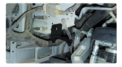
STEP 16 | The passenger side forward back mounting bracket will be mounted to the angled factory hole. Use a step drill to drill out the factory hole to 11/32" to accept an M6 riv-nut.
