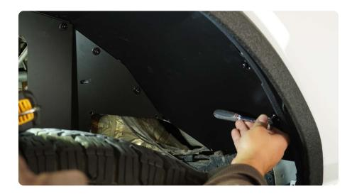
STEP 20 | Reach behind the inner fender and secure the M6 hex bolt for the forward back mounting brackets using a 10mm wrench.
