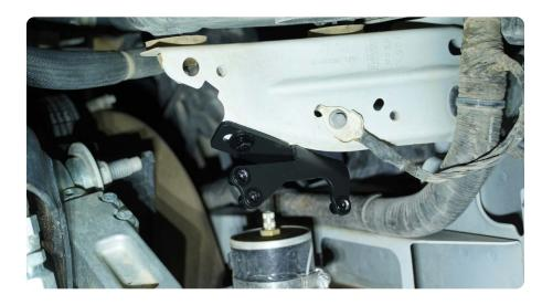
STEP 18 | Place the assembled DV8 inner fenders inside of the wheel well. Loosely mount the inner fender to the previously installed riv-nuts using the provided M6 hardware. Start all mounting bolts by hand first.
