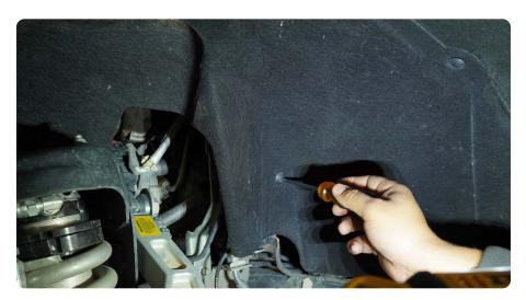
STEP 3 | Use a 7mm socket to remove the (6) hex head bolts that secure the inner fender to the fender.
