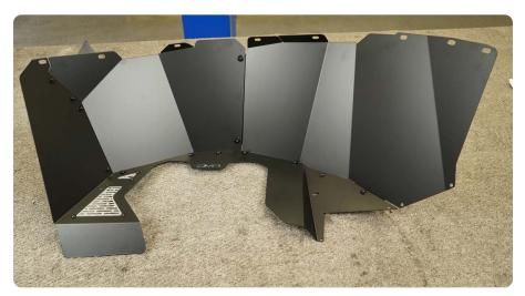
STEP 10 | If you are running factory suspension, place the small panel behind the base panel and large sized panel. Secure the base panel and large sized panel to the small panel using the provided M6 hardware.
