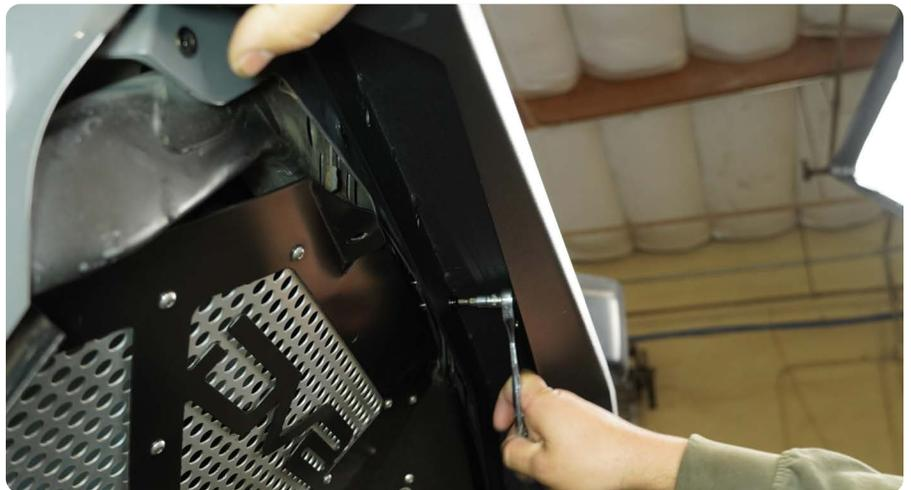
**STEP 15** | With all M6x20mm allen bolts started, secure the M6 hardware hand tight using a #4 allen tool.
