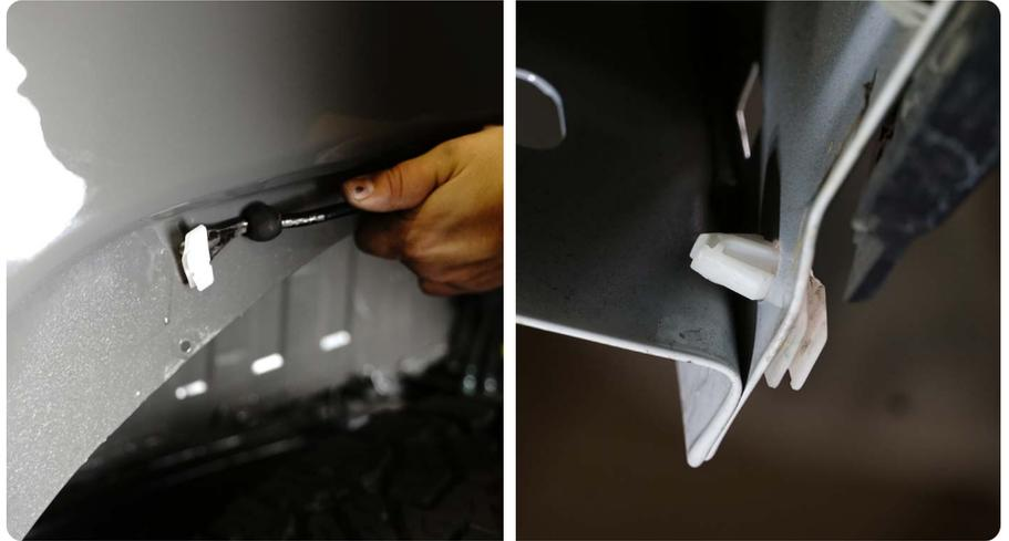
**STEP 8 |** Using your preferred cutting tool, cut the circled fender mounts off and grind them down so it is flush with the vehicle.
