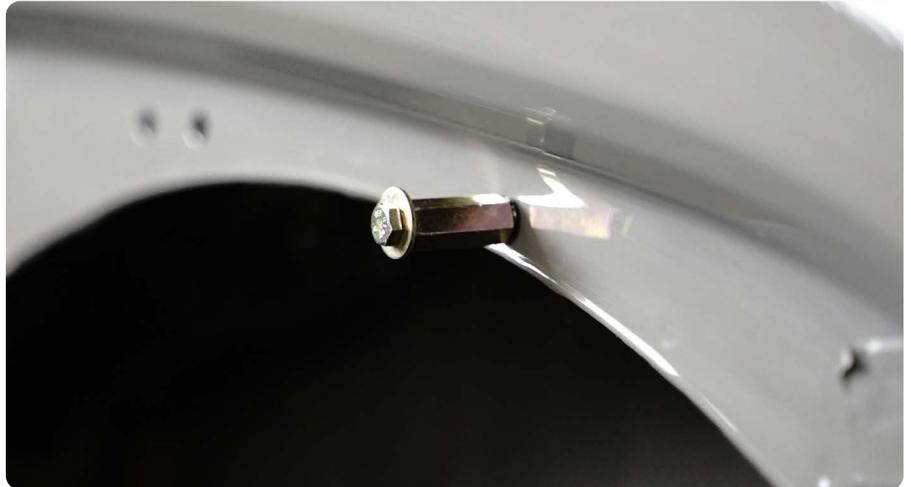
**STEP 27** | Use a 12mm wrench to hold the spacer while tightening with a 10mm socket. Tighten slowly until the nutsert is set properly. Do not over tighten.
