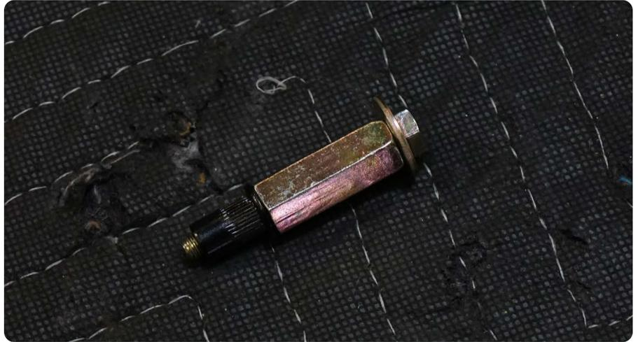
**STEP 26** | Slide the nutsert tool with the nutsert into the mounting hole. Ensure the flange of the nutsert is flat against the vehicle prior to tightening.
