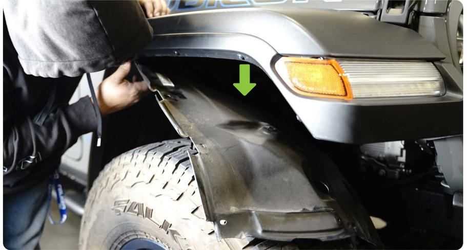
**STEP 2 |** Unplug the turn signal indicator by pulling the red release tab out and pushing on the black locking tab.
