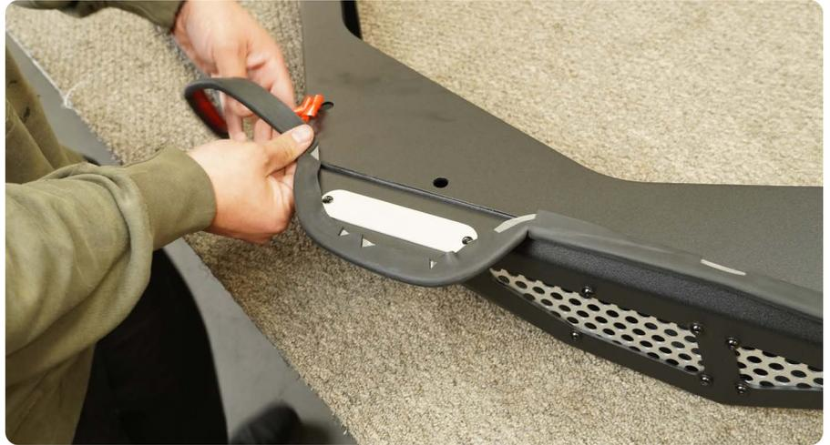
**STEP 12** | If planning to bypass vent cover, cut the seal at the fender corner. Continue the seal down the fender aligning the seal cut outs with the mounting holes in the fender. Cut off any excess seal.
