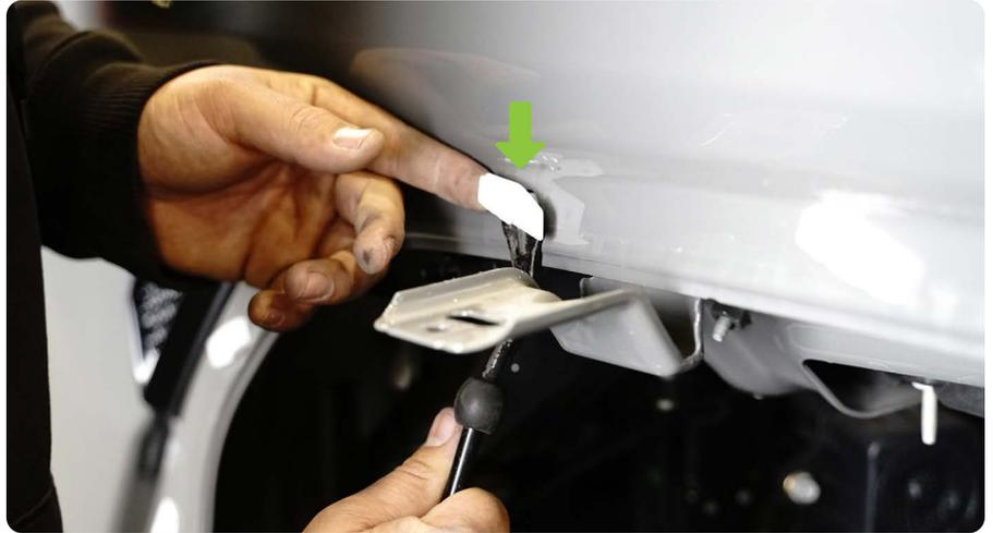
**STEP 5 |** (Rear uninstall) Use a 8mm socket to remove the bolts located along the interior of the inner fender.
