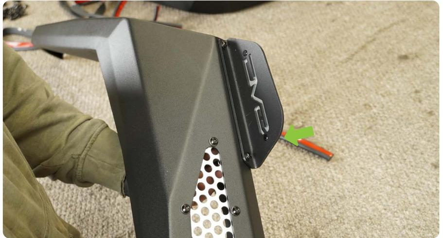
**STEP 11** | Place the peel-N-stick rubber seal onto the back of the fender, aligning the cutout in the seal with the fender mounting bolt holes.
