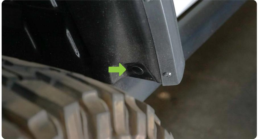
**STEP 6** | Remove the fender flare by pulling the front section towards the front of the vehicle, and the rear section towards the rear.
