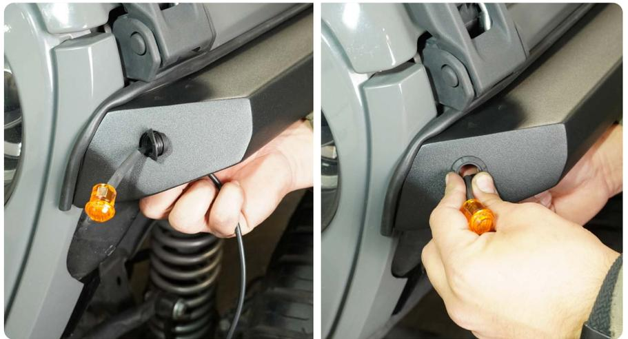
**STEP 17** | Press the marker light into the rubber grommet, route the marker light wiring harness behind the inner fender and connect plug it in to the vehicles factory fender/turn single light harness.
