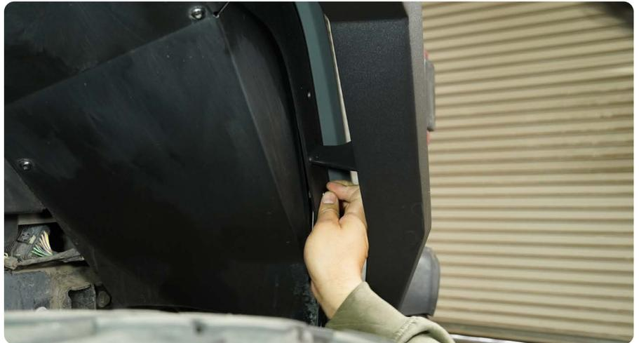
**STEP 23** | With all hardware started, secure the fender in place using a #4 allen tool.
