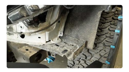
STEP 42 | To secure the inner fender, use a pick to poke a hole through the inner fender, using the factory welded nut as a guide.
