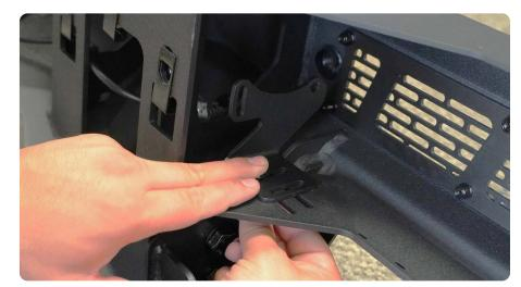
STEP 32 | Using the hardware provided with the light, install the light onto the brackets and secure the light to the brackets.
