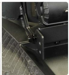
STEP 29 | Place the provided foam onto the mating surface of the bumper or wings as shown.
