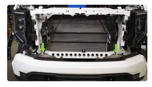
STEP 17 | Use a 15mm socket to remove the (6) bolts that secure the factory bumper mounting plate to the frame rails.
