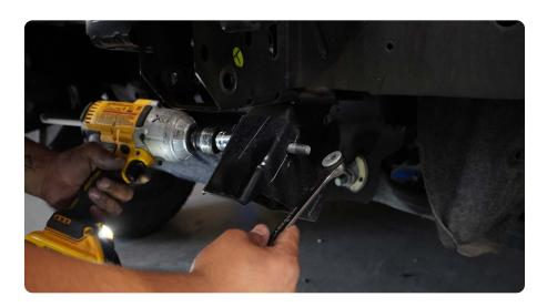
STEP 20 | Use a 10mm socket to remove both front inner fender supports.
