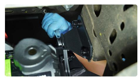
STEP 45 | Use a 18mm socket and an 19mm wrench to secure the M12 hardware.
