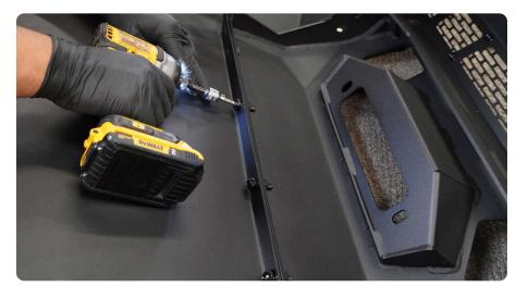
STEP 27 | If running a winch, use the hardware provided with the winch to install the winch onto the winch plate.
