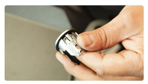
STEP 34 | Install the sensor bezels into the DV8 front bumper by pressing them into the bumper from the front side.
