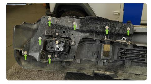
$\begin{array}{c|c} \text{STEP 23} & \text{Using a trim tool, remove} \\ \text{the clips holding the harness to the} \end{array}$ bumper.
