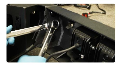
STEP 31 | If running a 20" dual row light behind the mesh, use the provided M6 hardware to loosely secure the provided brackets.
