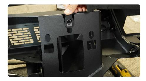
STEP 26 | Install the skid plate using a #6 Allen head and M8 Allen hardware. Ensure the bottom of the bumper and bottom of the skid plate are even.
